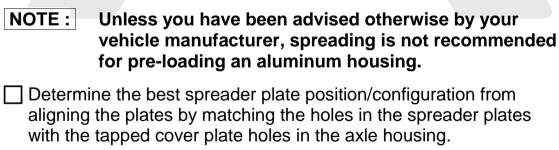
NOTE: Ensure that a large spreader pin hole in each plate is in line with the spreader sockets in the axle housing if sockets are available, and ensure that the plates are clear of all suspension components.
