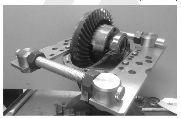
NOTE: Space the plates away from flange with flat washers if necessary.
